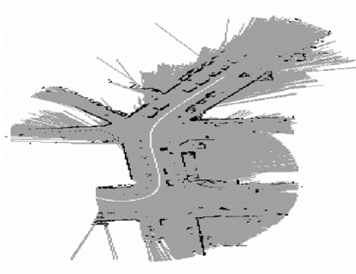
Figure 2: Occupancy grid and a planned trajectory
