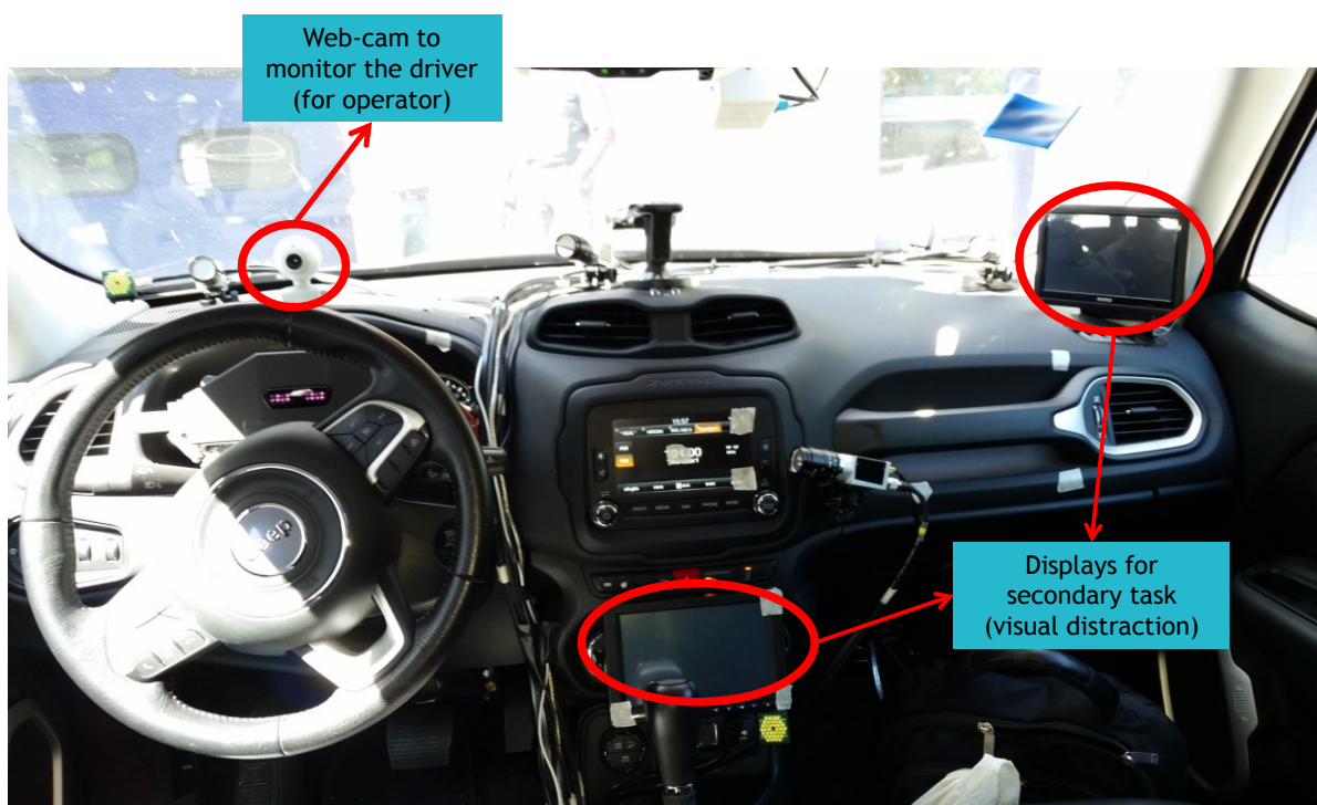
Figure 2: cockpit experimental installation
