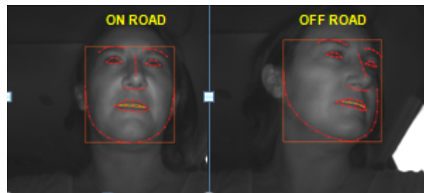
Figure 3: Classification of driver distraction states by the application based on the observed area
