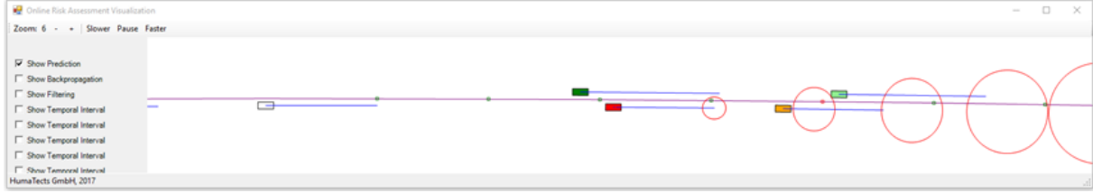
Figure 8: Screenshot of an exemplary visualization of the 95% prediction ellipses of the position of the lead vehicle (red). The coloured rectangles represent vehicles in the vicinity of the TeamMate vehicle (white rectangle). Blue lines indicate heading vectors, the purple line represents the centreline of a two-lane motorway.
