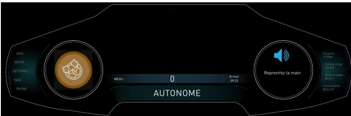
Figure 18 : The dashboard when a manual takeover is requested.
