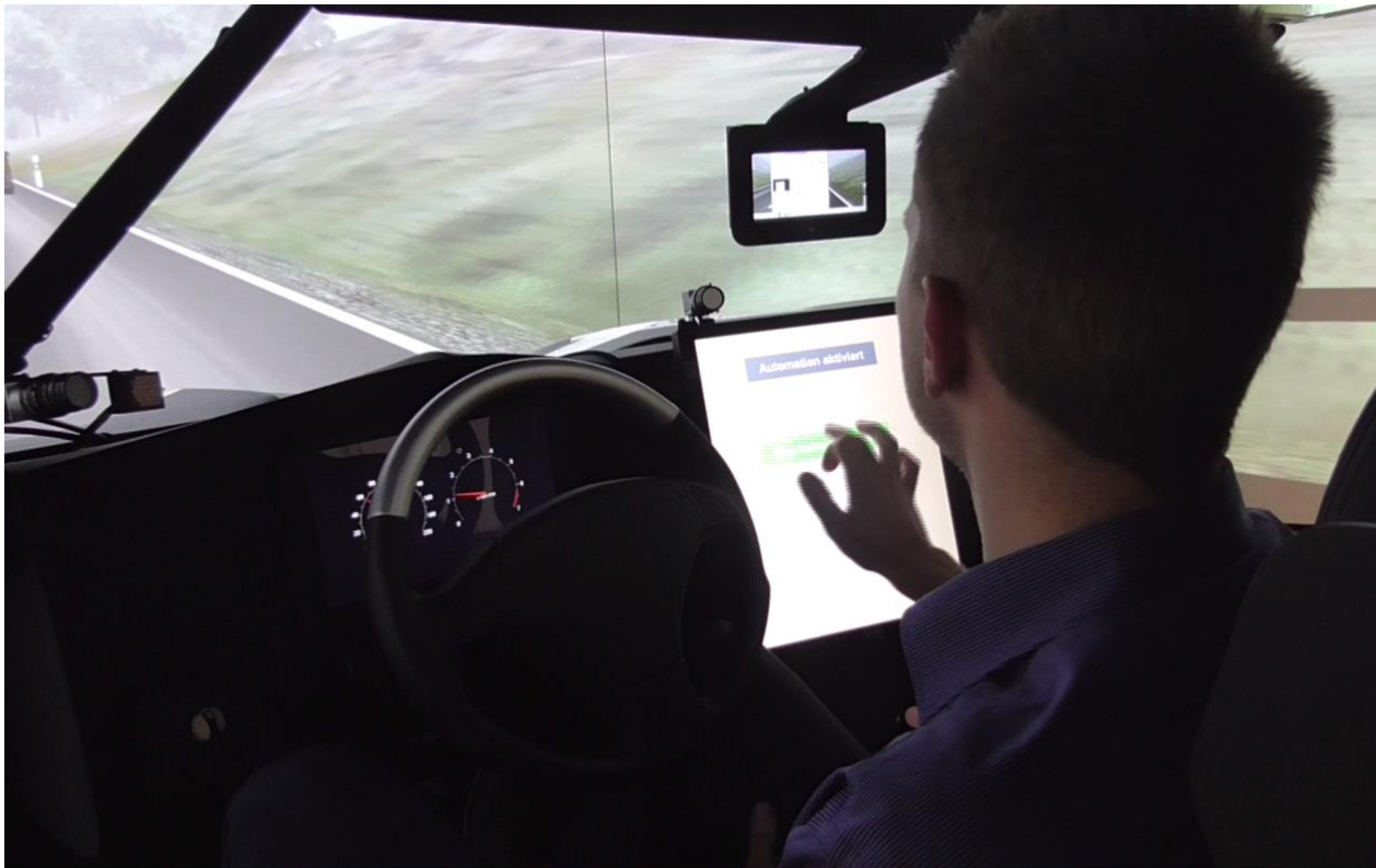
Figure 15: Touch screen with automation and overtake button
