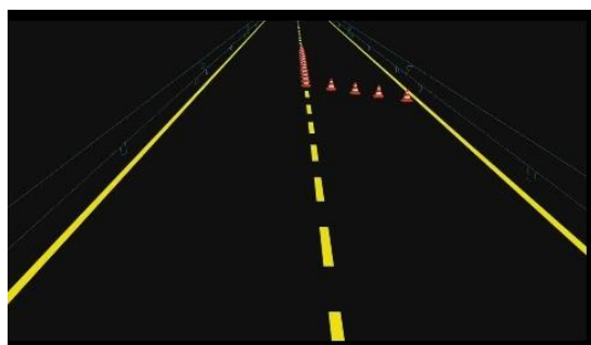
Figure 21: Pictogram symbolizing the roadwork zone displayed in the centre of the dashboard during the takeover request.
