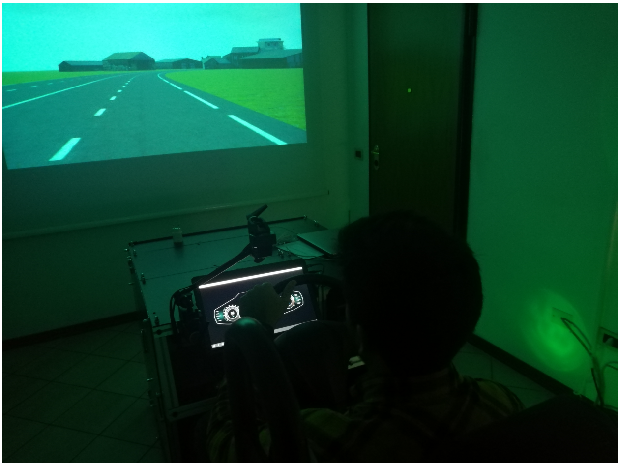
Figure 37: Experimental setup at REL driving simulator (with ambient lights)
