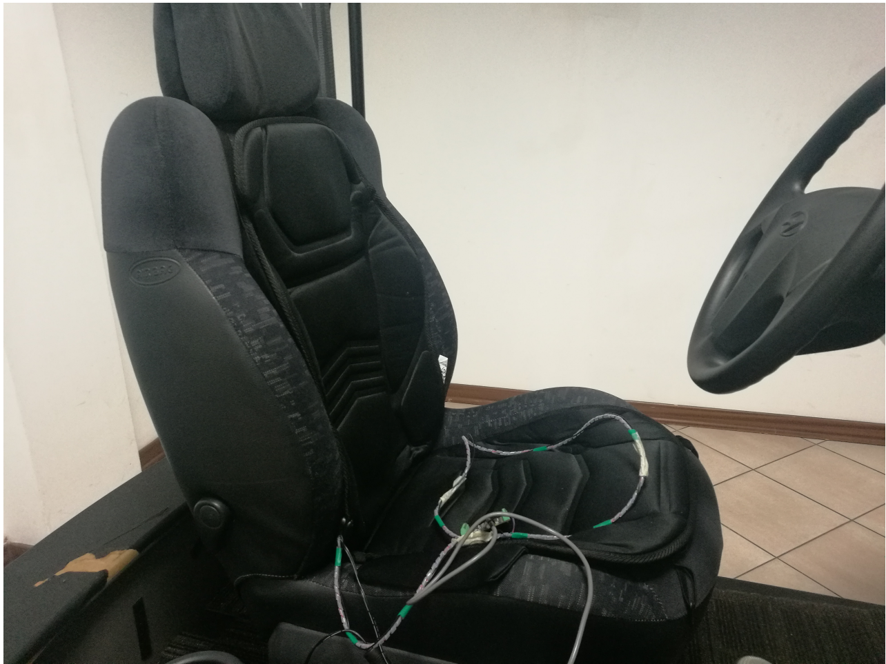
Figure 16: Haptic seat cover integrated in REL driving simulator
