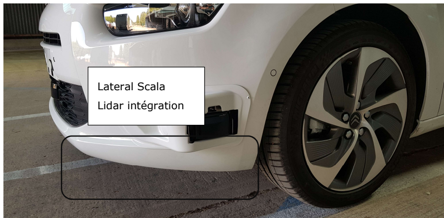
Figure 35: Lateral LiDAR integration.
