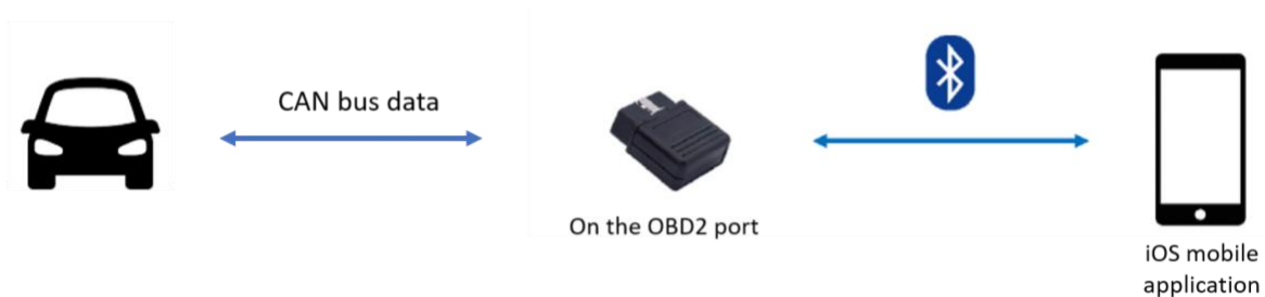
Figure 4: Overall architecture of the Mobile APP Extension SDK
